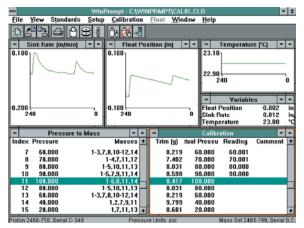
WinPrompt is acquiring information from the piston gauge through the piston gauge monitor and displaying it in real time. The data is being used to automatically adjust the pressure/mass values.
