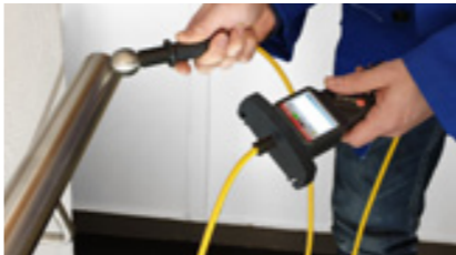
Testing of stair rails that protrude into the water
