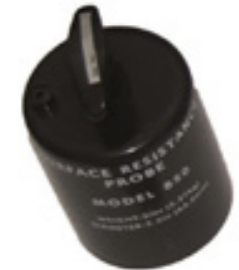
73012 Electrode for surface resistance
