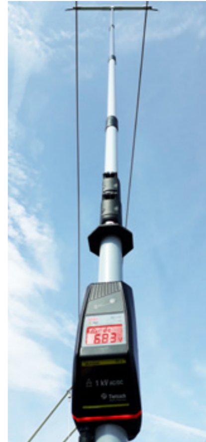
Variable test height up to 6,5 m and compact design thanks to telescope system in two sizes
