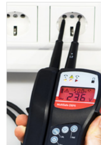
One-hand operation for testing sockets
