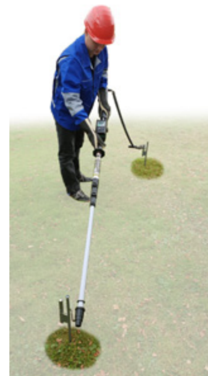
Check earth by second earth spike
