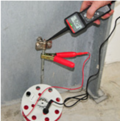
Quick compensation of the measuring line
