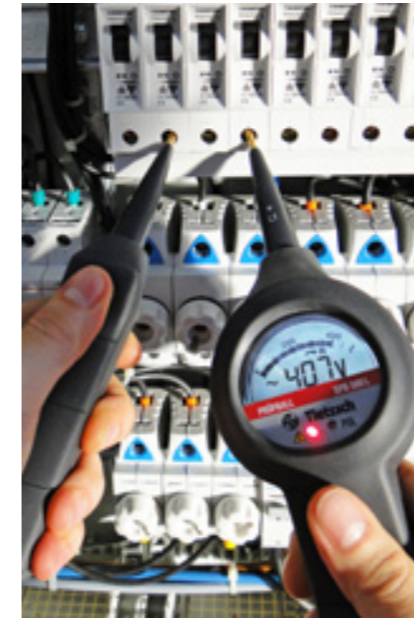
Direct voltage indication without pressed buttons
