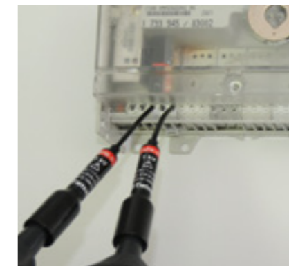
Flexible pin prods for tight contacts
