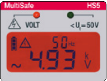
Colour change of the display at voltage
