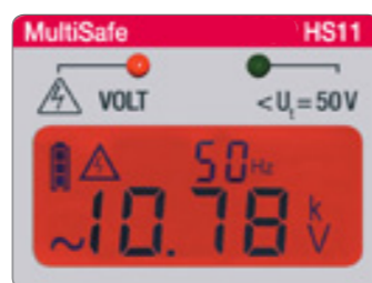
Colour change of the display at voltage
