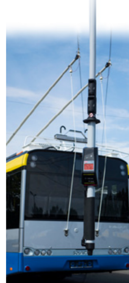
Clear indication of voltage by LCD, LED and acoustic signal.
