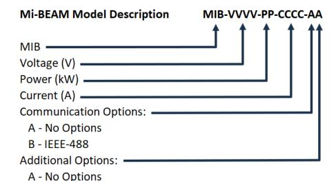
Note: The Mi-BEAM has a Universal 3-Phase AC Input to accept 200VAC to 480VAC (Range 180VAC to 528VAC).
