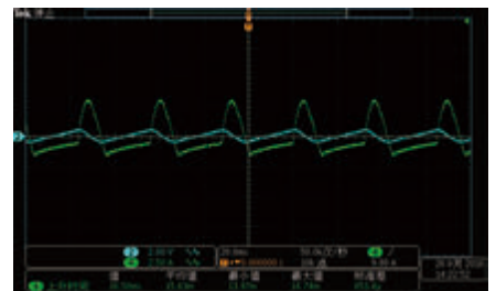
CV 50V low speed mode: it's obvious to find vibration phenomenon
