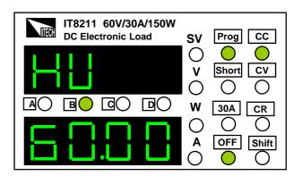
6) Press view key to enter Low Voltage setting. use cursor keys and the knob to set the low limit of the input voltage. Right figure set the Low Voltage as 0.00V.
