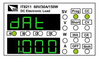
4)Press **Cview** key to enter Delay Time setting, use cursor keys **△ B** and the knob **o** to set the delay time, the range of a single step is 0.4s to 25s. Right figure set the DT as 5s.
