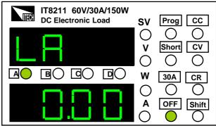
11) When past the test successfully, the instrument display as normal; when fail to pass the test, the instrument will display as right figure, display wrong step, alarm 3 second and shut the input. Right figure show the condition the first step not pass.
