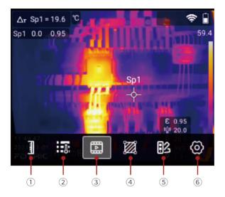
① **Temperature scale:** Auto scale, Manual scale, Touch scale settings.
