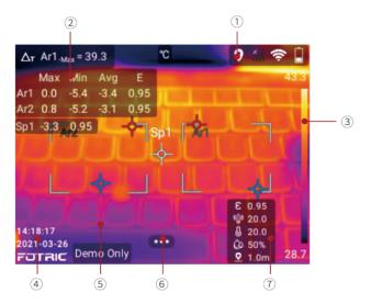
① **Status Bar:** Display Battery, Wi-Fi, Bluetooth, GPS, TF card low storage warning, Laser warning etc.
