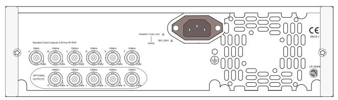
The frequency standard signals are available at the BNC-connectors on the rear panel. The rear panels of 908 and 909 are identical. This picture shows the 909 version incl. Option 70 (11 BNC-outputs).
