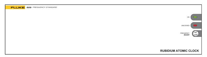
Front panel of 909. The ON indicator shows when power is connected. The UNLOCK indicator warns when the output frequency is not yet locked to the rubidium element. The adjustment potentiometer is located under the calibration seal.
