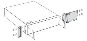
• Fasten the 908 or 909 in the rack via screws in the four rack mounting holes
