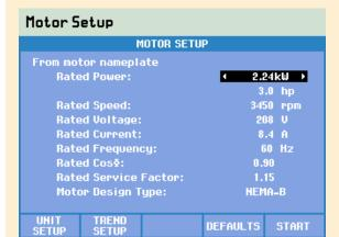
Input details of the motor from the rating plate including rated power, rated speed and motor type from either NEMA or IEC classifications.
