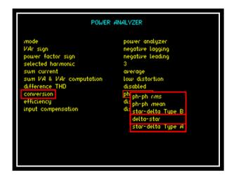
It is not possible for the instrument to detect the wiring configuration used to connect the instrument to the motor / DUT. All "conversion" options have to be available with the User ensuring the correct option is selected from the menu.
