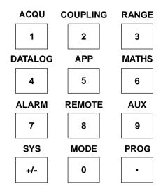
SELECT MENUS for non-mode-specific configuration. Also use as numeric keypad when entering parameter values or data.
