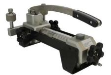
The CP582 Hydraulic High Pressure Test Pump is a hand operated pressure pump designed to generate pressure from 0 to 70MPa (10,000 psi). It is simple operation and achieves high pressure smoothly and easily. The pre-pressuring hand pump can fill large volume workload quickly. A hand tight vernier control allows the high pressure to be easily generated and controlled smoothly.
