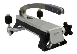
The CP577 uses a unique dual stage pump design where a low pressure, high volume chamber is used to pre-charge a secondary high pressure chamber. This allows the pump to reach high pressure quickly and with a minimal amount of effort. The pump motion stays smooth through the entire stoke. A precise Vernier control allows pressure to be fine turned with high resolution. The Vernier chamber provides enough range so it can be used to generate low pressure 500mbar with no pumping.
