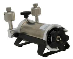
The Model CP571 low pressure calibration pump is a low air pressure source with the ability to easily adjust and stabilize. This hand pump possesses a pressure range of  $\pm$  40kPa; uses air as the media, and can adjust the pressure easily and stably.
