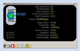
Real-time visual monitoring of piston gauge parameters with ready/not ready indication is possible in COMPASS when used with interfaceable devices.
