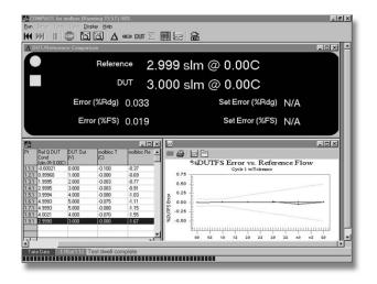
While running a test, complete operating information is available through six display windows that can be turned on/off and scaled at will. These include real time readings from the molbox and the DUT, calculated errors and deviations, error plotting and a point by point data grid. The current test definition and DUT profile can be accessed by clicking icons.
