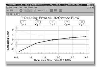
A PLOT function is also included to generate a variety of detailed error plots from data files. Extensive customization is supported. The plots can be created, viewed and printed.
