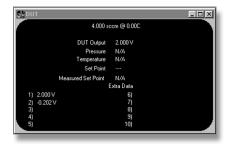
After the last test point, the flow is set to zero and a comment field is presented for entering comments specific to the test. The comments are stored with the test data file.
