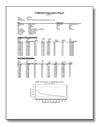
COMPASS includes a Report Editor to allow final, formatted test reports to be produced within the COMPASS environment. The Report Editor is template based. Several standard templates are included. Custom templates can be created from scratch or by editing existing templates. All the data file variables as well as COMPASS plots can be embedded into the template.
