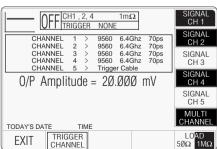
Whenever the DC waveform is selected within the DC/Square function an extra Soft Key is available in the CHANNEL SELECT sub menu.
