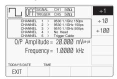
Pressing first the required ratio, then 'EXIT' returns to the trigger selection screen. On this screen, no indication of the trigger ratio is given.
