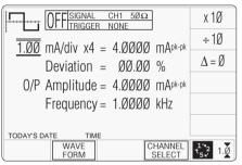
The above default screen has auto-selected the symmetrical square waveform, as indicated by the icon in the top left corner. Frequency is variable between 10.000Hz and 100.00kHz. Frequency has defaulted to 1kHz, deviation  $^{\prime}\Delta^{\prime}$  to zero, and output current to 4.0000mAp-p. The Duty Cycle is fixed at a nominal 50%.
