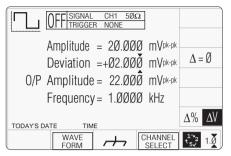
Fig. 4.4.10 Voltage Deviation Applied
