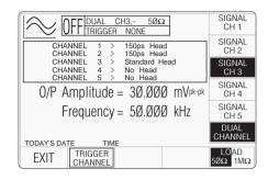
Next select the Slave channel, in this case Signal Channel 2:
