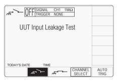
The above default screen has auto-selected the open-circuit output, as indicated by the icon in the top left corner, and the highlighted screen key on the bottom row.
