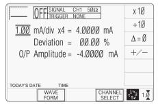
Once into DC function, it is not necessary to change the waveform to change polarity. Pressing the +/- screen key toggles between positive and negative DC Current. The polarity selection is shown by the function icon in the top left corner, confirmed by the + or - sign on the O/P Amplitude value.
