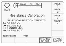
Note that the other 9500B functions, listed in paras 10.2.3 and 10.2.4 cannot be externally adjusted during Mainframe calibration (they are either derived directly from functions that can be calibrated, or are calibrated 'for life' during manufacture, or are adjusted during 'Head' calibration). Attempting to select these functions during Mainframe calibration, while the Model 9500B is in CAL mode, will result in an error message being displayed:
