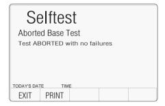
If there were no failures up to the point of aborting, this is shown on the screen.
