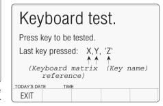
The 'Keyboard matrix reference' (X,Y) relates to the electronic matrix which is used to transfer keypress information to the internal processor, and does not relate closely to the physical layout of keys. The 'Key name' (Z) is the name, in words, which describes the last key to be pressed.
