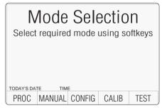
Press the CONFIG screen key at the center of the bottom row to progress into 'Configuration' mode. The 9500B will transfer to the open 'Configuration' information screen:
