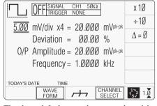
The above default screen has auto-selected the positive square waveform, as indicated by the icon in the top left corner. Frequency is variable between 10.000Hz and 100.00kHz. Frequency has defaulted to 1kHz, deviation  $^{\prime}\Delta^{\prime}$  to zero, and output voltage to 20.000mVp-p. The Duty Cycle is fixed at a nominal 50%.
