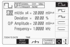
The WAVEFORM key label is highlighted to indicate that waveform selection is available, as is the presently-selected waveform icon. Pressing one of the waveform keys (for example: the key) to select a different
