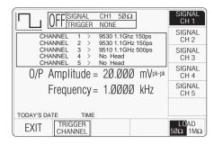
As can be seen from the screen, Model 9530 heads are fitted to channels 1 and 2, a Model 9510 head is fitted to channel 3, and no heads are fitted to channels 4 and 5.
