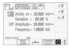
Fig. 4.3.3.2 Manual Mode Power-Up Screen — Multi-Channel
