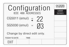
Note that the 9500B contains two IEEE-488 interfaces, each of which will respond to a separate address. 9500B and CG5011 occupy one IEEE bus address and can be modified either on the 9500B screen or the 5000 series screen. SG5030 occupies the other bus address, which can be modified only on the 5000 series screen. The 5ØØØ SERIES selection also switches the interface to accept the emulation commands only.
