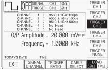
The expected load value can be changed from  $50\Omega$  to  $1M\Omega$  using the bottom left corner toggle key.
