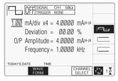
Both polarities of DC Current output are listed merely as different waveforms. As an example, pressing the \_\_\_\_\_ key from the setup shown above will present the DC function screen, showing negative values selected (of course, the frequency parameter has disappeared from the screen):
