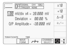
Once into DC function, it is not necessary to change the waveform to change polarity. Pressing the +/- screen key toggles between positive and negative DC Voltage. The polarity selection is shown by the function icon in the top left corner, confirmed by the + or - sign on the O/P Amplitude value.
