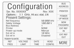
provide entry to a second 'Configuration' menu screen, showing the present settings of other parameters. *Refer to para 3.4.3.14*.
