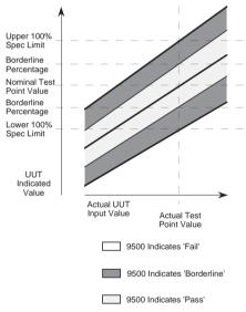
When in Procedure mode, the direct-printing certificate (Style 1), and the data on the 'Results' card, will report 'Borderline' test results. Users have access via Configuration mode to set the percentage for borderline reporting.
