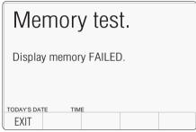
If a failure is reported, rectification will require access to the internal circuitry, so no further user action is recommended, except to report the result to your Fluke Service Center.
