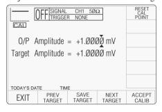
This screen initially shows the value to which the 9500B output is presently set, and the value of the selected target amplitude (whether 'default' or 'saved'). Note that on these values, triangular cursors indicate which digit will change when using the cursor keys or spinwheel. When transferring, using the 'tab' \( \) key, the cursor always moves to the least significant digit on the other value.
