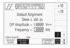
The above default screen has auto-selected 'Default Alignment', as indicated by the top line of text and the highlighted screen key on the bottom row. The unequallized (default) alignment has a maximum skew of ±50ps between channels. The amplitude and default frequency are also shown on the screen.
