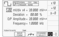
Fig. 4.4.1 Typical Screen in Scope Mode
