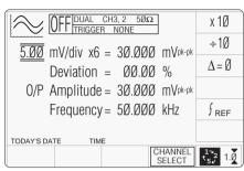
Note that the upper sinewave amplitude range limits are halved by invoking Dual Channel Sine function.
