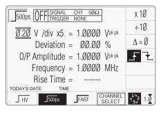
The above default screen has auto-selected a frequency of 1MHz, a rise time of 500ps, zero deviation and an output level of 1Vpk-pk.
