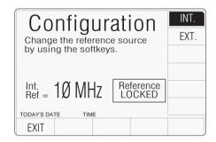
3. When switched to 'EXT.', use the up/down cursor control or spinwheel to inform the 9500B of the source frequency. Ensure that the required source is connected and operating.
