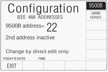
The 9500B IEEE-488 bus address can be set to any number within the range 0 to 30.
