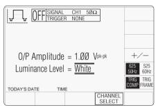
The above default screen has auto-selected 625 lines / 50Hz and triggers will be from composite video. Amplitude has defaulted to a luminance level of 'White' at 1.0V p-p.
