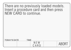
In this case, insert the card required for the UUT into PCMCIA SLOT 1, push gently home, and press the 'NEW CARD' screen key for the sequence to continue.
