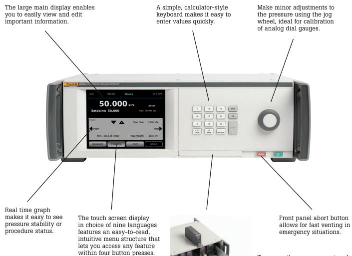
To access the measurement and control modules, simply open the front panel. Modules are easy to replace, even when the 8270A or 8370A is rack-mounted.
