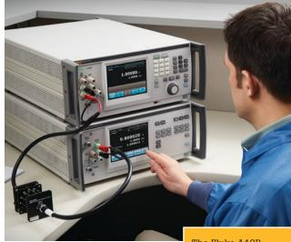
The Fluke A40B expands the capability of the 5790B to allow you to make very precise absolute and relative current measurements You no longer need to calculate the current value, allowing you to perform calibrations more quickly with less potential for errors.
