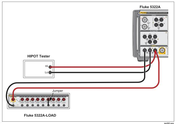
Figure 64. Normal Hipot Calibration Connections for Voltages <1100 V
