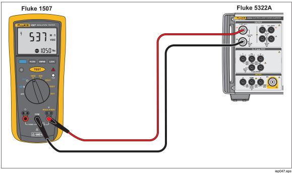
Figure 33. Calibrating Insulation Resistance of a Handheld Insulation Tester
