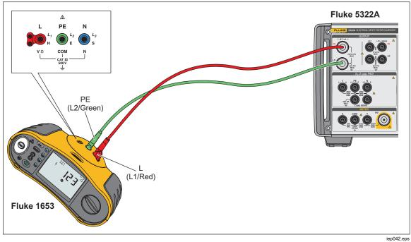
Figure 52. Voltage Calibration on Battery-Powered Installation Testers
