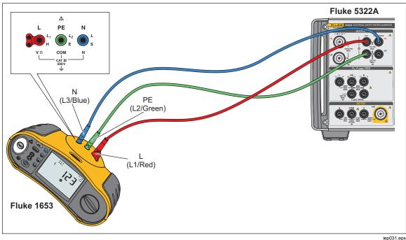
Figure 31. Earth Resistance Calibration Connections
