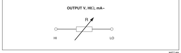
Figure 11. Simplified Substitute Leakage Current Schematic
