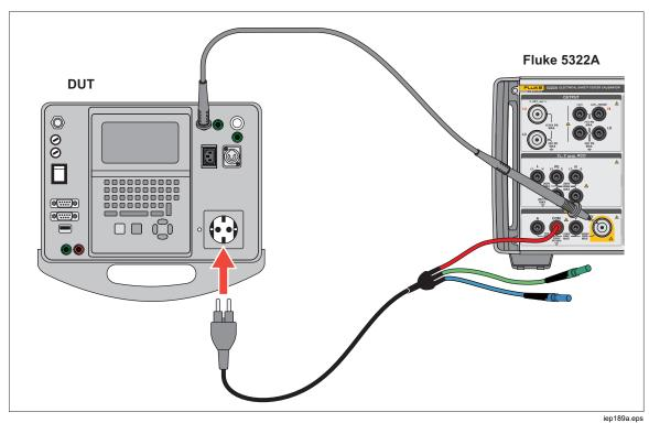
Figure 58. Class II Flash Test Voltage Measurement using the Flash LC Mode
