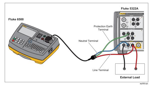
Figure 55. Voltage and Current Meter Calibration with a Cable Adapter
