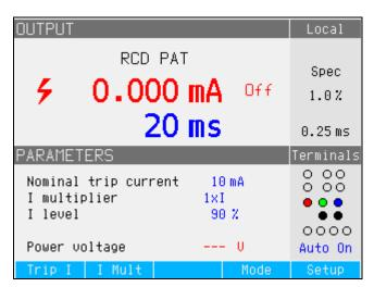
Figure 18. Calibrating RCD Trip Time in PATs
