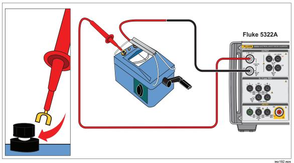
Figure 36. Hand Crank Insulation Tester Connections
