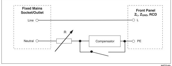
Figure 7. Simplified Loop Impedance Source Schematic
