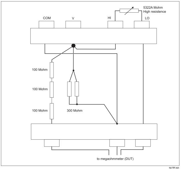
Figure 40. Internal Resistance Multiplier Option Connection
