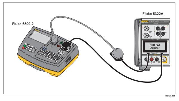
Figure 50. RCD in PAT Connection with the RCD PAT Adapter
