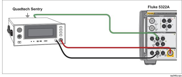
Figure 60. 5 kV Internal Probe Application
