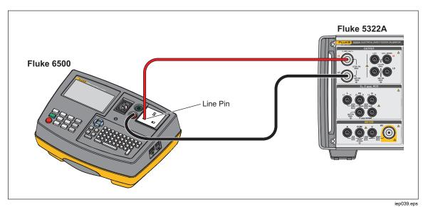
Figure 46. Touch Leakage Current Calibration on Fluke 6500
