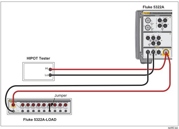
Figure 65. Normal Hipot Calibration Connections for Voltages >1000 V
