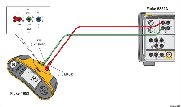
Figure 30. 2-Wire Resistance Calibration DUT Connections
