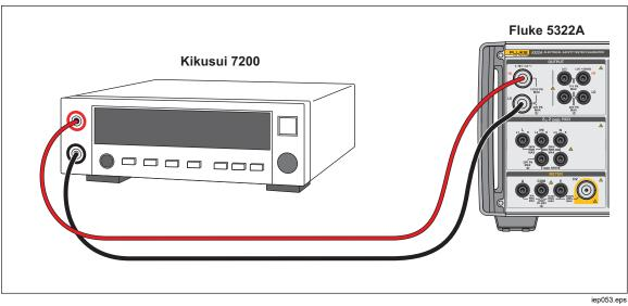
Figure 35. Calibrating Insulation Resistance of an Electrical Safety Analyzer
