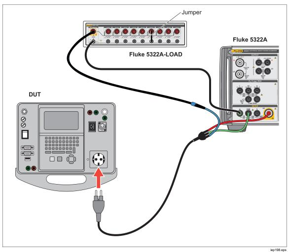
Figure 59. Class I Flash Leakage Current Measurement
