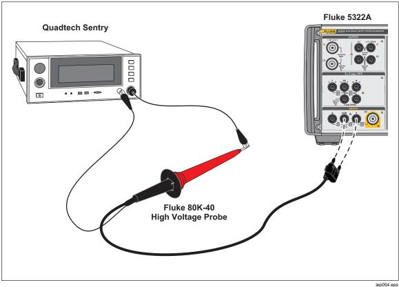
Figure 62. 40 kV High Voltage Probe Application
