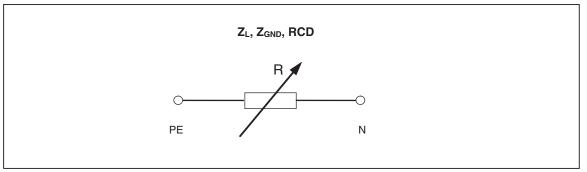
Figure 5. Simplified Ground Bond Resistance Source
