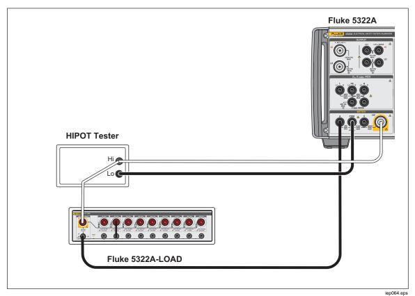
Figure 25. HIPOT LC Function Connections for >1100 V and up to 5000 V rms
