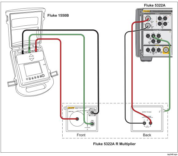
Figure 38. Connections to 1550B when using Resistance Multiplier
