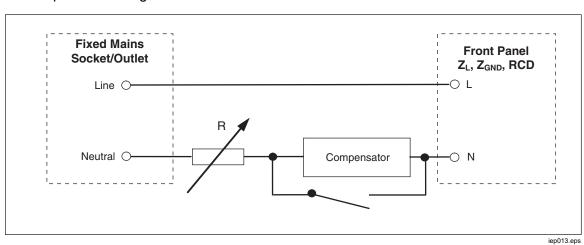
For line impedance calibration, an internal resistance is inserted between the N terminal on the front panel and the Neutral of the power line input on the rear panel. See Figure 6.
