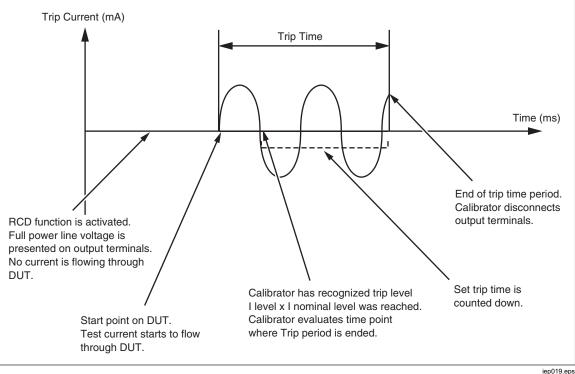
Figure 14. RCD Trip Time Process
