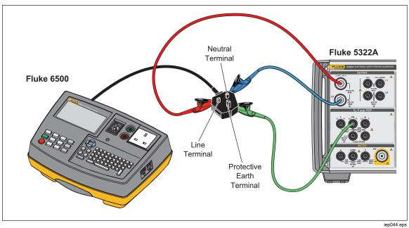
Figure 54. Voltage Calibration using Single Wires
