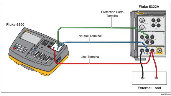
Figure 56. Voltage and Current Meter Calibration with Single Wires
