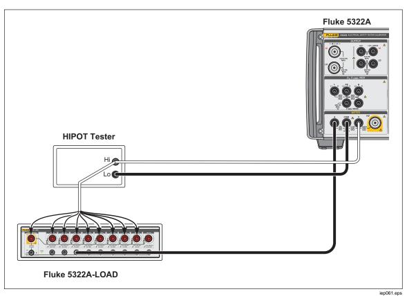
Figure 24. HIPOT LC Function Connections for <1100 V
