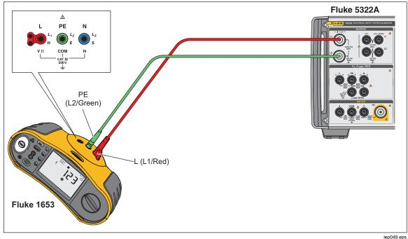
Figure 32. Calibrating Insulation Resistance of an Installation Tester
