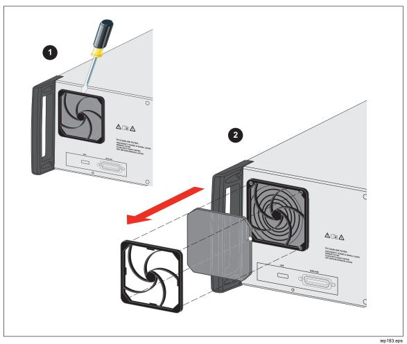
Figure 29. Remove the Air Filter
