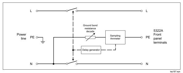
Figure 12. Simplified RCD Scheme
