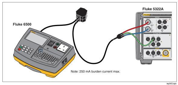
Figure 53. Voltage Calibration on Line Powered Appliance Testers
