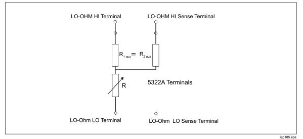
Figure 3. Simplified Low Resistance Source Schematic
