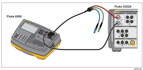
Figure 34. Calibrating Insulation Resistance of a Portable Appliance Tester
