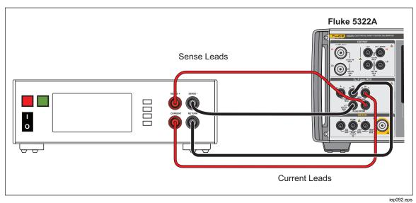
Figure 43. Ground Bond Resistance Calibration on Bench Ground Bond Tester
