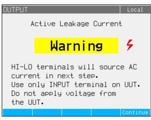
Figure 10. Active Leakage Current Warning Message
