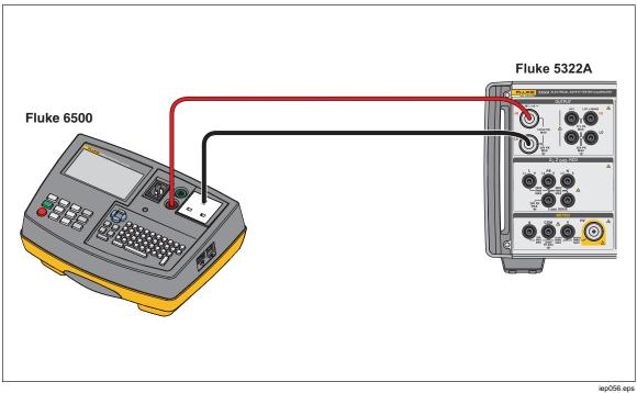
Figure 47. Active Leakage Current Calibration on Fluke 6500
