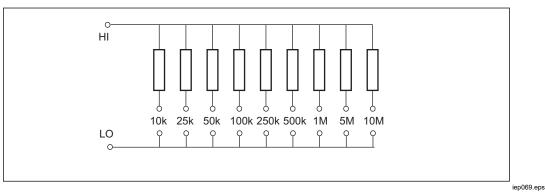
Figure 63. Load Schematic
