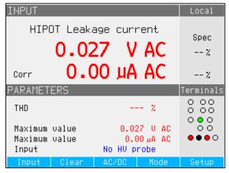
Figure 23. Multimeter Display with Hipot Leakage Current Measurement for Voltages <1100 V
