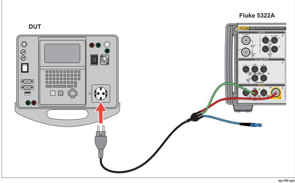
Figure 57. Class I Flash Test Voltage Measurement
