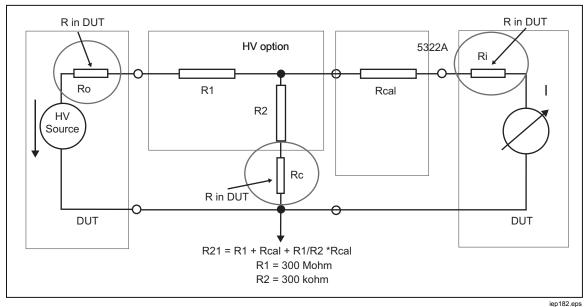
Figure 41. Sources of Error when Using the Resistance Multiplier
