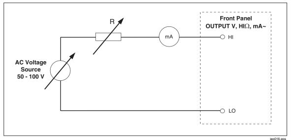
Figure 9. Simplified Active Leakage Current Scheme
