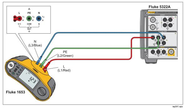
Figure 49. RCD Trip Time and Trip Current Calibration
