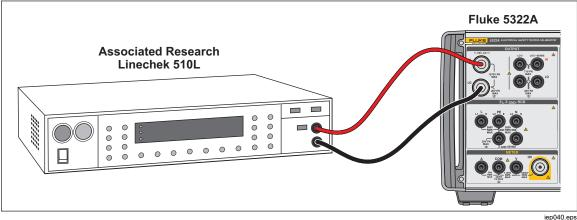
Figure 48. Leakage Current Calibration on Earth Leakage Tester
