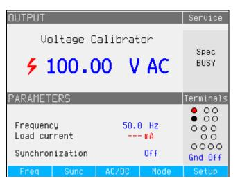
Figure 20. AC Voltage Calibrator Display
