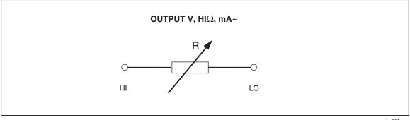
Figure 4. Simplified High Resistance Source Scheme
