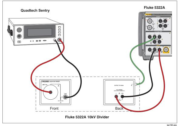
Figure 61. 10kV Divider Application
