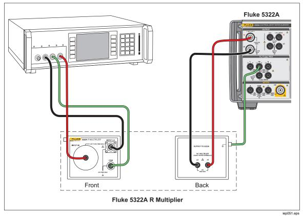
Figure 37. Connections to Bench Tester when using Resistance Multiplier Adapter
