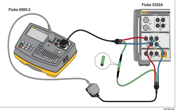
Figure 51. RCD in PAT Alternate Connection
