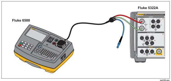
Figure 45. Passive Leakage Current Calibration on Fluke 6500
