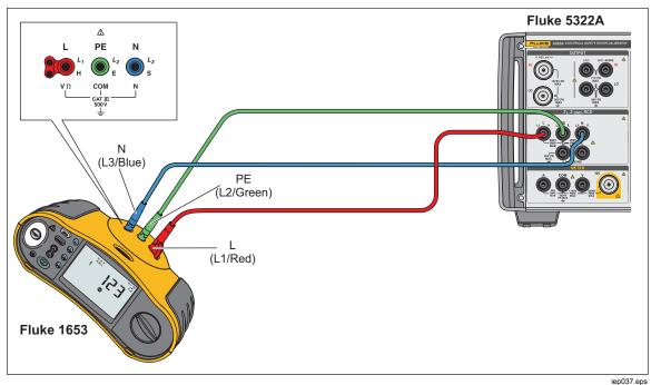
Figure 44. Line and Loop Impedance Calibration on a Fluke 1653
