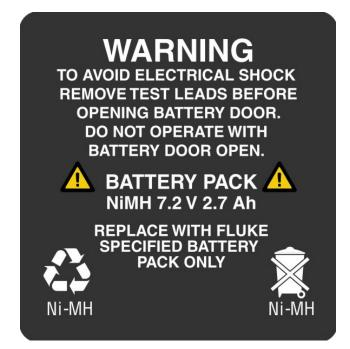
Figure 1-2. Instrument Labels
