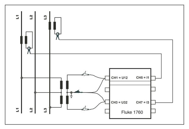
Figure 3-3. Circuit Diagram: Aron 2 Method/Open Delta Method
