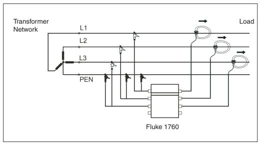
Figure 3-4. Circuit Diagram: 4-Wire Network (Wye Connection)
