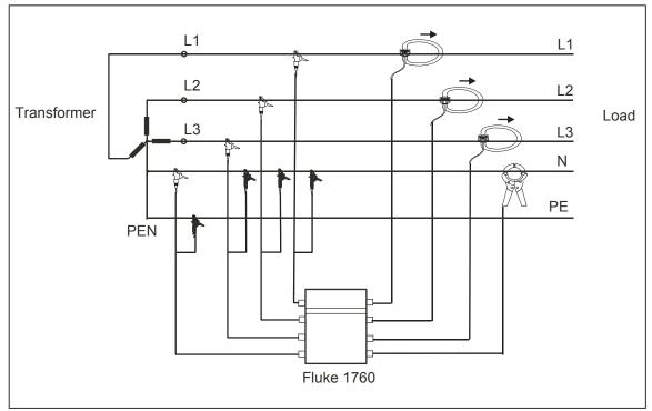
Figure 3-5. Circuit Diagram: 4-Wire
