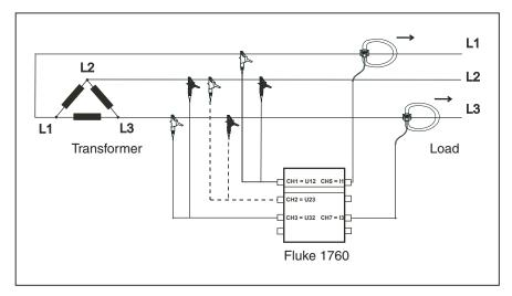
Figure 3-2. Circuit Diagram: 3-Wire Network (Aron 2)
