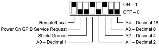
Figure 2–1. SFA Configuration Switch
