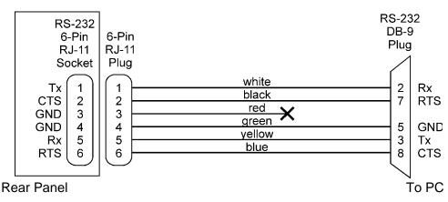
Figure 2–3. SF to PC RS-232 Connection (RJ-11 to DB-9)
