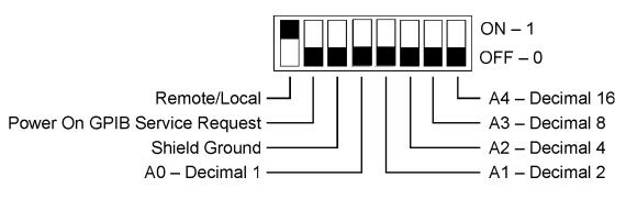
Figure 2–2. SFI Configuration Switch
