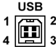
Figure 3-11: USB Connector pin orientation.
