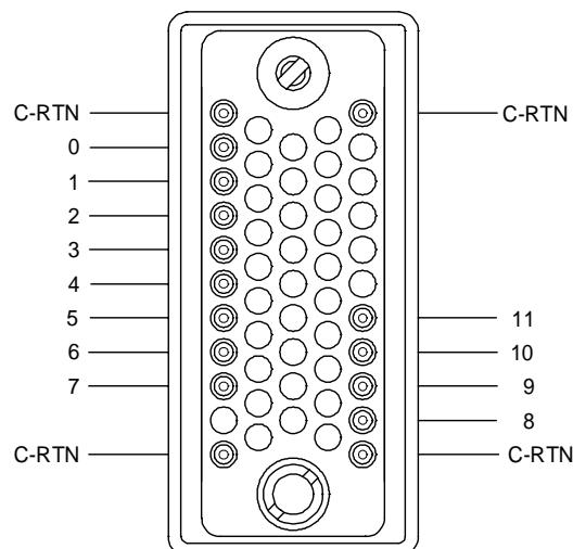
C-RTN is connected with the Modul-GND and the shield
