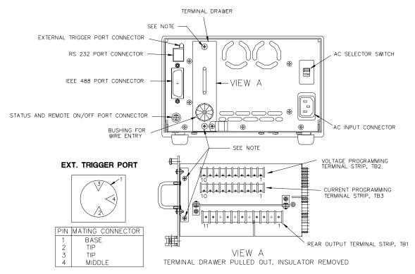
NOTE: REMOVE SCREWS AND PULL OUT DRAW TO ACCESS REAR OUTPUT TERMINALS AND VOLTAGE AND CURRENT PROGRAMMING TERMINALS
