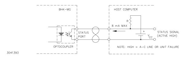
FIGURE 2-7. STATUS PORT OPTO-COUPLER ACTIVE "HIGH" CONFIGURATION
