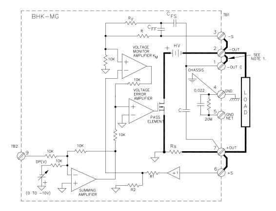
NOTES: 1. UNIT SHOWN IN SLOW MODE, LOCAL SENSING. REMOVE LINK BETWEEN TERMINAL 1 AND 2 FOR FAST MODE.
