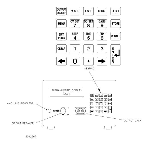
FIGURE 2-1. BHK-MG SERIES, FRONT PANEL CONTROLS, INDICATORS AND CONNECTORS
