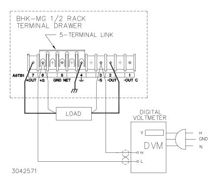
FIGURE 2-5. REMOTE SENSING, FAST MODE SELECTED, POSITIVE OUTPUT GROUNDED
