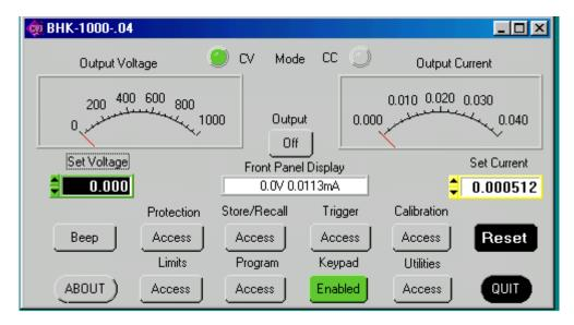
FIGURE 4-2. MAIN PANEL (BHK 1000-40MG, TYPICAL)
