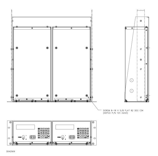
FIGURE 1-3. RA 24 RACK ADAPTER WITH TWO 1/2 RACK BHK-MG 40W UNITS
