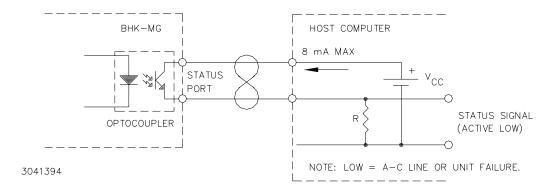
FIGURE 2-6. STATUS PORT OPTO-COUPLER ACTIVE "LOW" CONFIGURATION
