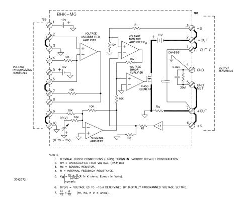
FIGURE 3-7. ANALOG VOLTAGE PROGRAMMING, SIMPLIFIED DIAGRAM
