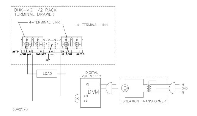
FIGURE 2-4. LOCAL SENSING, SLOW MODE SELECTED, GROUNDING NETWORK CONNECTED, FLOATING OUTPUT (FACTORY DEFAULT CONFIGURATION)
