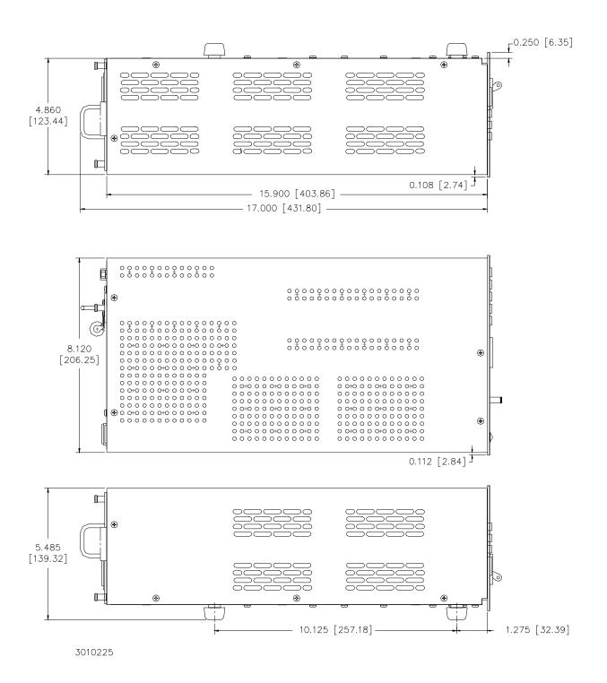
FIGURE 1-2. BHK 40W SERIES POWER SUPPLY, MECHANICAL OUTLINE DRAWING (SHEET 2 OF 2)
