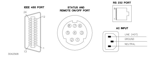
FIGURE 2-2. BHK-MG SERIES, REAR PANEL CONTROLS AND CONNECTIONS
