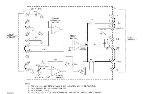
FIGURE 3-8. ANALOG CURRENT PROGRAMMING, SIMPLIFIED DIAGRAM
