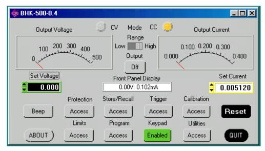
FIGURE 4-2. MAIN PANEL (BHK 500-0.4MG, TYPICAL)
