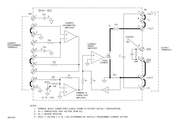
FIGURE 3-8. ANALOG CURRENT PROGRAMMING, SIMPLIFIED DIAGRAM
