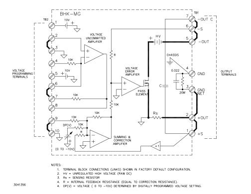
FIGURE 3-7. ANALOG VOLTAGE PROGRAMMING, SIMPLIFIED DIAGRAM
