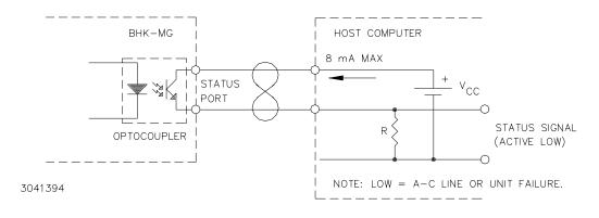
FIGURE 2-7. STATUS PORT OPTO-COUPLER ACTIVE "LOW" CONFIGURATION
