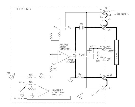
NOTES: 1. UNIT SHOWN IN SLOW MODE, LOCAL SENSING. REMOVE LINK BETWEEN TERMINAL 6 AND 7 FOR FAST MODE.
