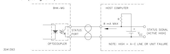
FIGURE 2-6. STATUS PORT OPTO-COUPLER ACTIVE "HIGH" CONFIGURATION
