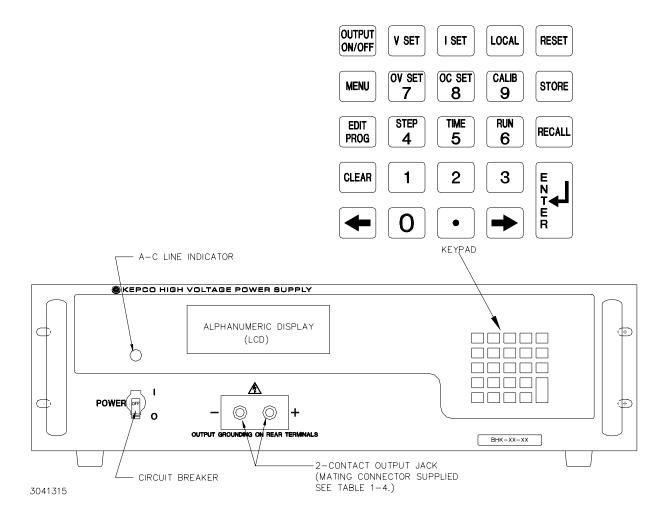
FIGURE 2-1. BHK-MG SERIES, FRONT PANEL CONTROLS, INDICATORS AND CONNECTORS
