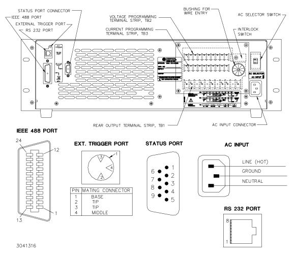
FIGURE 2-2. BHK-MG SERIES, REAR PANEL CONTROLS AND CONNECTIONS
