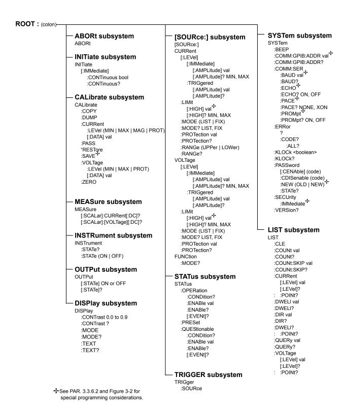
FIGURE 3-5. TREE DIAGRAM OF SCPI COMMANDS USED WITH BHK-MG POWER SUPPLY
