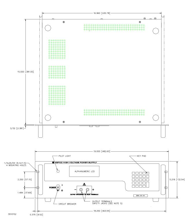
FIGURE 1-2. BHK SERIES POWER SUPPLY, MECHANICAL OUTLINE DRAWING (SHEET 1 OF 2)
