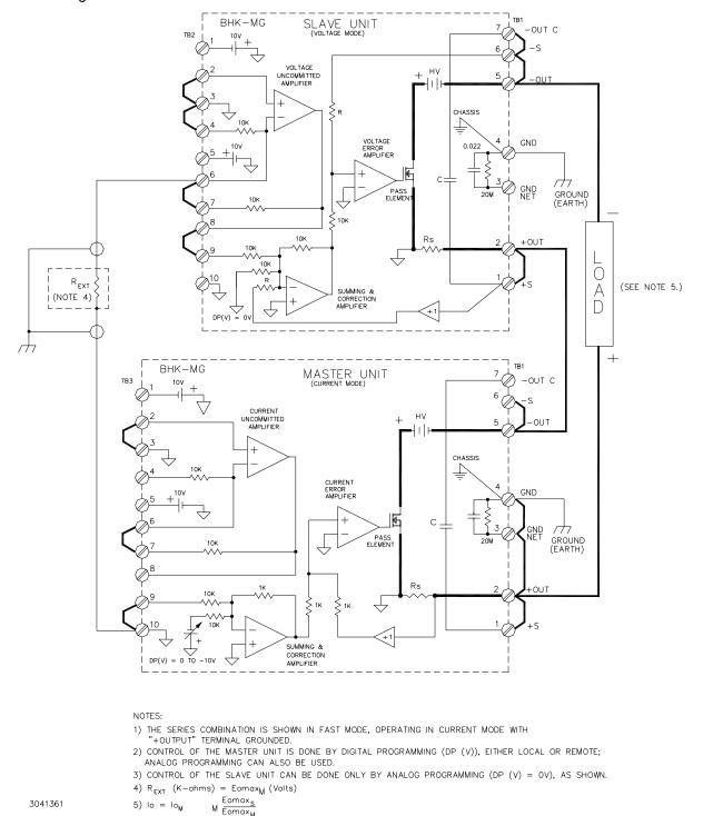
FIGURE 3-22. SERIES MASTER-SLAVE (CURRENT MODE) CONFIGURATION
