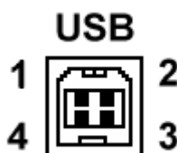
Figure 3-6: USB Connector pin orientation.
