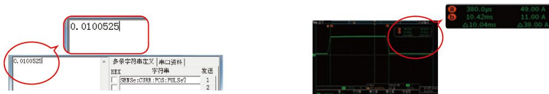
Fig 3. Time Measurement Comparison between IT8900A and oscilloscope
