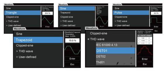
Users can also edit waveforms through the interface's customization mode to mimic and reproduce the real power waveforms at the scene of the problem.
