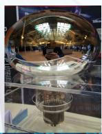
iseg PHQ modules are developed as direct HV supply of modern photo multiplier tubes (PMT) with the high voltage power supply integrated in the PMT socket. Advantages of PMT-integrated power supplies are:
