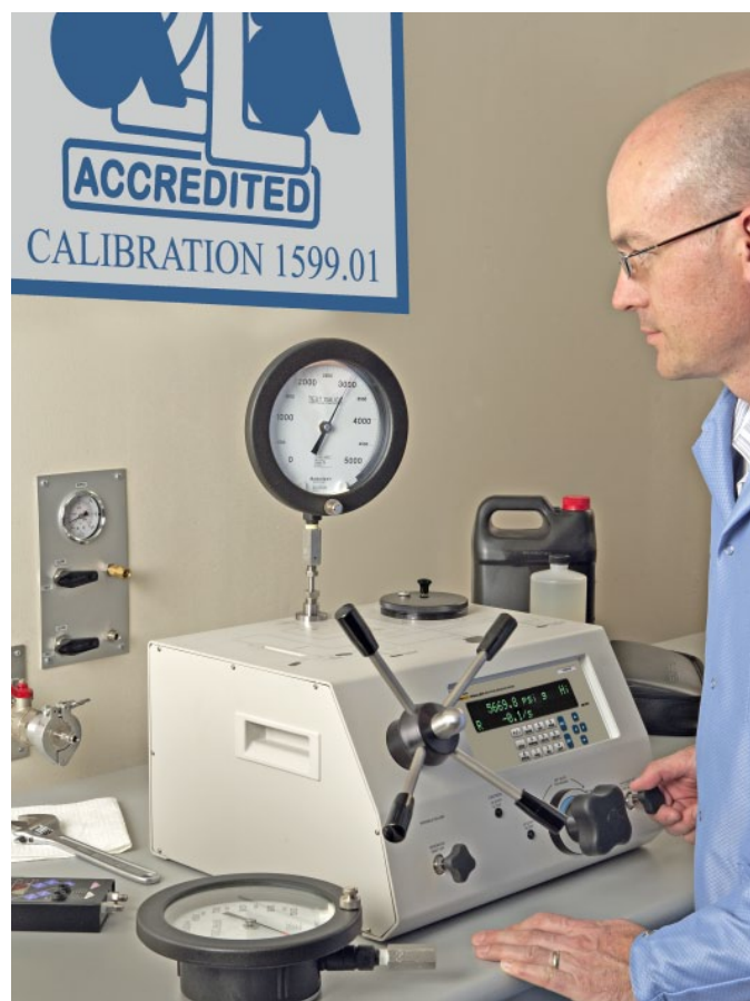
E-DWT-H's fine adjustment valve enables the operator to set pressure to the exact nominal value on the gauge under test.
