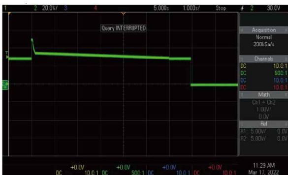
LDC302 28V abnormal voltage transients (overvoltage)
