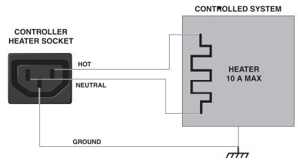
Figure 1. Controller to Heater Wiring
