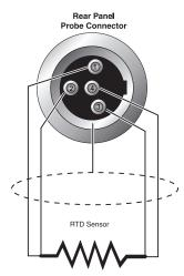
Figure 2. RTD Probe Wiring
