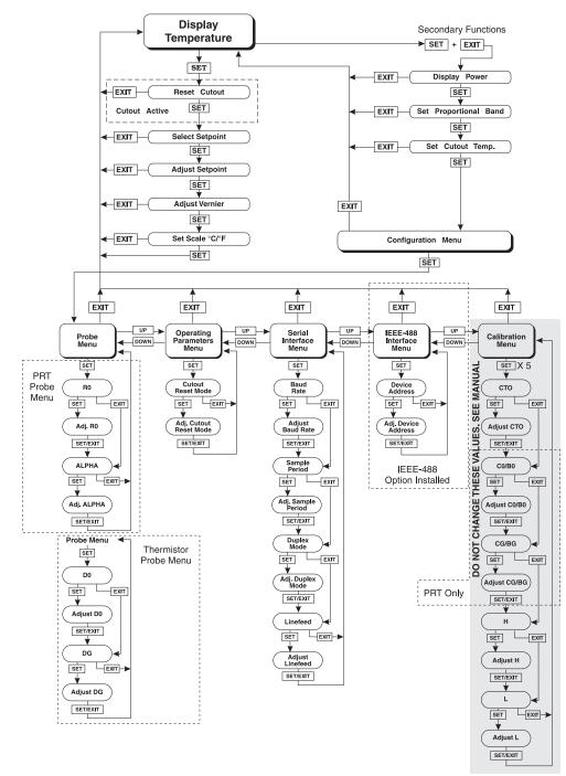
Figure 6. Controller Operation Flowchart
