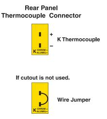
Figure 3. Cutout Probe Connections
